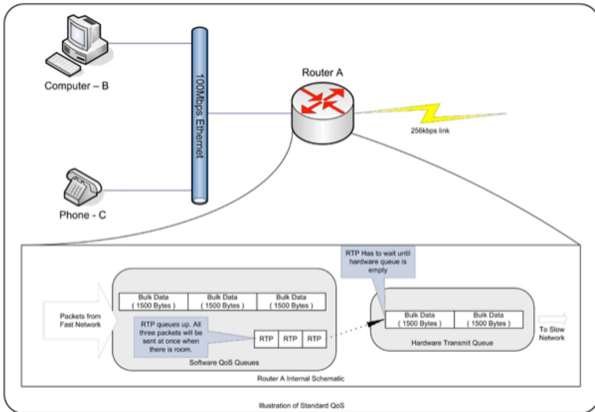
Data enters the router (A) from a 100Mbit/s LAN interface. A computer (B) on the LAN is sending an e-mail with a large attachment, and since the LAN is 100Mbit/s his computer sends many large (typically 1500 byte) packets to router A in quick succession.
